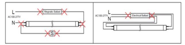
Third Step: Install the LED tube, and make the electrical connection.
