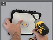
Replace white reflector using existing slotted mounts.
