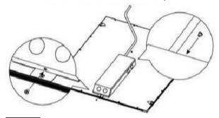
STEP4 Adjust panel Light to Fit the Ceiling Frame
