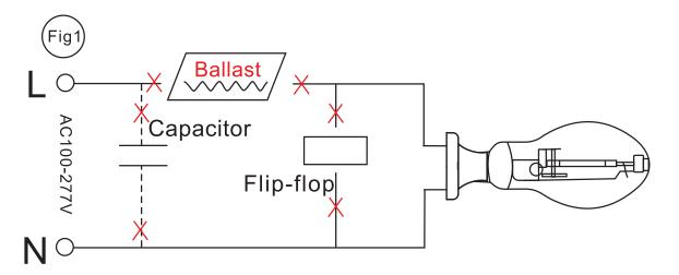
2. Reconnect directly to the existing lamp holder. Shown as Figure 2 (North America 100-277VAC)
